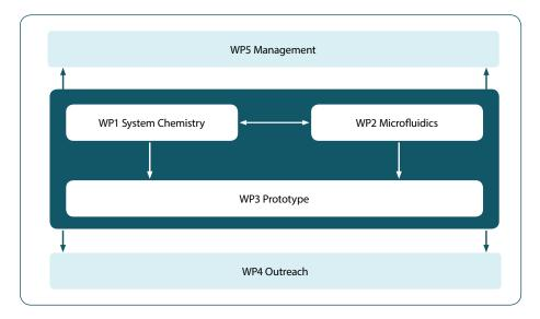
The first two WPs will start simultaneously, establishing the chemistry of a series of peptide hybrids (WP1) and developing microfluidic flow reactors (WP2). Starting in month 13 of the project, WP3 will develop a prototype of a cell-like molecular assembly line. WP4 and WP5 will be continuously ongoing for the entire project duration to ensure its smooth management and effective communication of its results.
